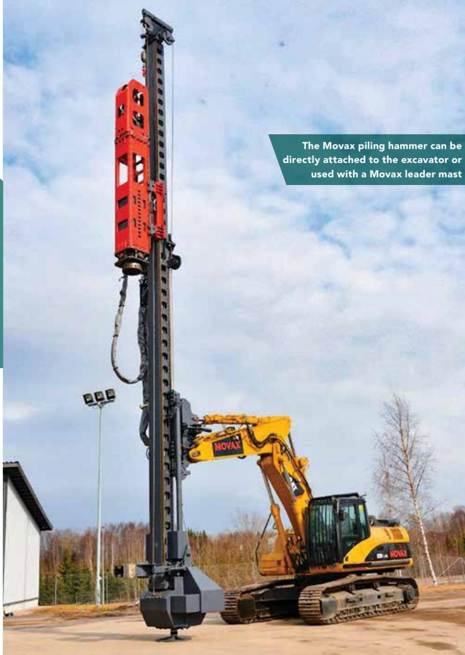
The Movax piling hammer can be directly attached to the excavator or used with a Movax leader mast
